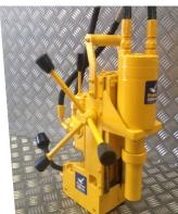
The HUW 150 Magnetic Drill was designed and developed for undersater use. This machine uses hydraulic power and a special mechanically switched magnet. It can cut very accurate holes through metal more quickly than traditional twist drills by only removing the material at the periphery of the hole being cut, leaving a solid slug which is ejected at the end of the cut. Capable of drilling clean, accurate holes up to  $60 \text{mm} \ \emptyset$  in metal and up to  $75 \ \emptyset$  thick.
