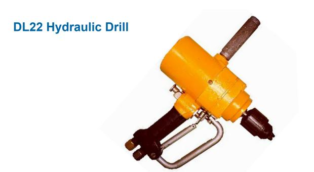
The DL22 is a portable hydraulic drill completely sealed for underwater operation. This drill delivers 240 rpm @ 11 l/min and up to 830 rpm @ 38 l/min Maximum torque output is 81Nm. There is also an insant reverse capability. The drill has a 3JT Jacobs chuck with 20mm capacity.
