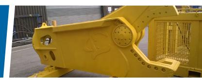
The 1344Te Hydraulic Shear is a versatile tool capable of performing fast and efficient scrap cuts on a variety of different grade materials of varying size and thickness.
