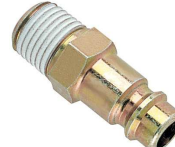
IB8NMC3 88103304 IBN/IBS Series nipple, 3/8" male thread, 8 mm bore (ISO6150B / MIL-C4109)
