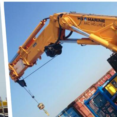
The AKC 145 LHE4 comes complete with a dedicated HPU, transport base with incorporated seafastening plates. Benefiting from dual control local and Canbus remote control allows the operation of the crane both from the dedicated operator's seat and also on deck ensuring best line of sight at all times.
