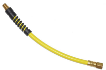
33104 91486330 Hose whip, 1/4" NPT, 6 mm inside diameter, 30 cm (1 ft)
