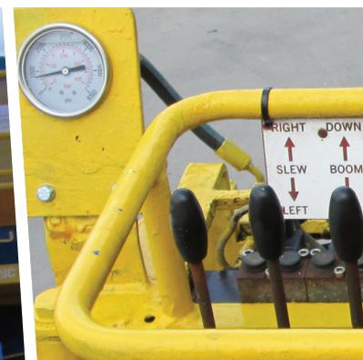
**The Effer 120000-3S Marine Crane comes complete with skid assembly suitable for deck mounting and electric hydraulic power pack.**
