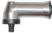
03070216 1/2" right-angle head (speed reduction: 25% torque output reduction: up to 50%)
